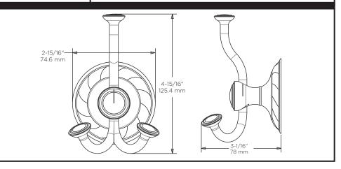
MATERIALS: Post and Hook - Zinc Die Cast Wall Plate - Steel, Nickel Plated
