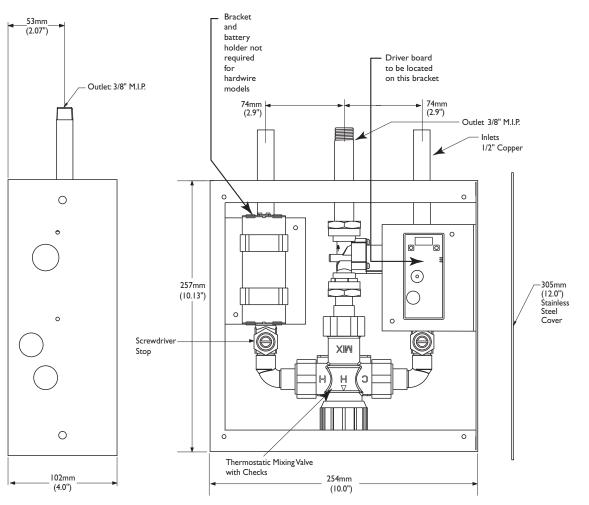
Note: For wallhung sink installations, sensor conduit rough-in should be directly under basin to minimize sensor cord exposure.
