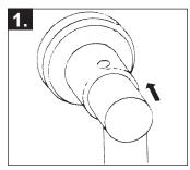
Place end mount of wall bar into the mount - do not tighten the set screw.
