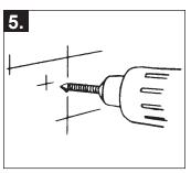
Drill hole for top mount. Use 1/4 inch carbide drill for ceramic tile.
