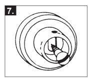
Secure mount to wall with screw. **Note:**Allen set screw must be at top of mount.
