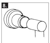
Place bar into mount. Do not tighten Allen set screw.
