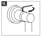
Tighten Allen set screw on both top and bottom mounts.
