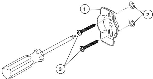
With the mounting bracket (1) oriented as shown, place it over the installed anchors (2) and install screws (3). Repeat for second mounting bracket.
