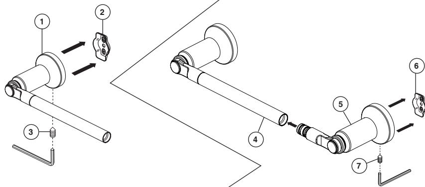
Position body (1) over mounting bracket (2) and tighten set screw (3). (Set screw should be on the bottom of body.) Place one end of the towel bar (4) into the second body (5), and place the other end of the bar into the first body (1). Slide the second body over the other mounting bracket (6) and tighten set screw (7).
