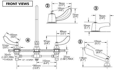
\* CAN BE CUT IN FIELD TO 152mm (6.0") MINIMUM INLET FOR 3/8" OR 1/2" FLEXIBLE RISER OR 1/2-14 NPSM COUPLING NUT (NOT SUPPLIED)
