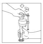
Replace cap by engaging lugs and rotating cap 1/8 turn clockwise.
