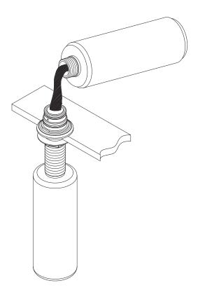
6. Put the pump nozzle and plastic pump into sleeve.
