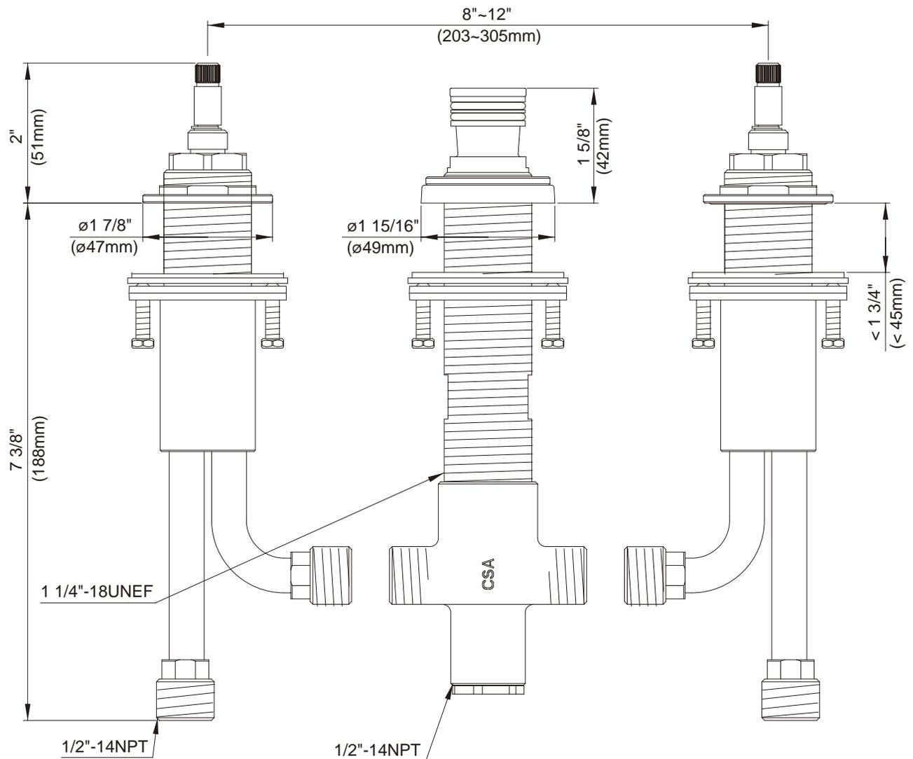
\* Installation method shown is for deck thickness of less than 1-3/4".
