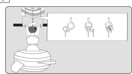
Lift fan onto the mounting bracket (#1). Turn housing until hanging ball seats itself into ball socket (listen for click).
