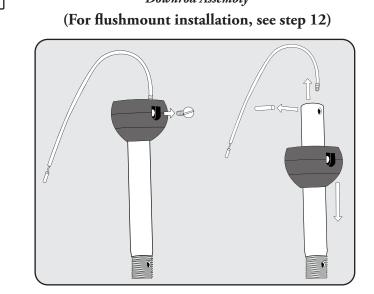
Locate downrod assembly (#2). Loosen ball screw on black hanging ball to free lock pin. Black hanging ball will slide down. Remove ground screw and green ground wire. Remove hanging ball from downrod and save all parts. Insert fan wires through downrod.
