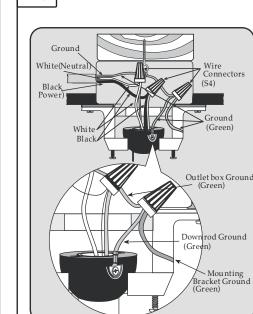
wires: white fan wire to white outlet wire, black to black and green to green. Wire connectors (S5) are provided for your convenience. 2. After connections are made, turn splices upward and push carefully into outlet box. Separate black wires on one side of the box, and white and green wires on the other side.
