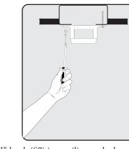
Prior to securing mounting bracket, screw "J" hook (S7) into ceiling outlet box as a secondary support means. Secure mounting bracket (#1) to the outlet box (A) by tightening bracket screws & washers (S2) as shown. If not mounting to an outlet box, use wood screws (S1) and washers (S1) and mount securely to ceiling beam. Be sure at this point to insert canopy screws in bracket.
