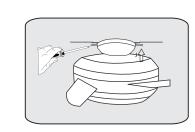
Remove three larger alternating screws from the coupling of the motor, align the holes of the bottom of the canopy and secure the canopy to the motor by using three screws previously removed. Hang the motor assembly onto the hook from the bracket allowing it to hang freely and connect the fan wires, as shown in step 10.
