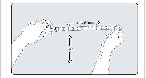
• Check to make sure blades are at least 30" from any obstruction. • Check Down rod Length to make sure blades are at least 7' above the floor.
