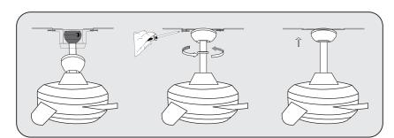
Loosen two screws from the hanger bracket and remove the other two. Align the canopy up to ceiling and over the loosened screw. Place the canopy into the key hole. Secure the canopy by tightening the previously loosened and removed screws. Attach canopy ring (#4) to canopy, press and lock into place.
