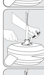
Insert saftey bolt (S6) through flange & downrod and attach nut. Tighten firmly.
