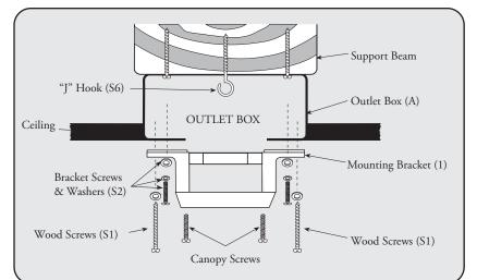
NOTE: Do not mount directly to sheet rock or ceiling tile.
