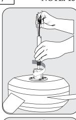
Thread the downrod onto the motor housing making sure the wires don't get twisted.
