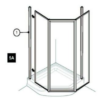
5B-5C. Engage the other side of assembly into wall jamb(#1)
