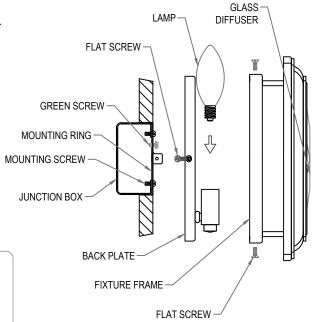
3. Fasten the white fixture lead to the white wire in the junction box. Fasten the wires together with an approved fastener (wire nut). Starting about 1" below the fastener, tightly wrap the connection with electrical tape so that the connections seals the end of the fastener.
