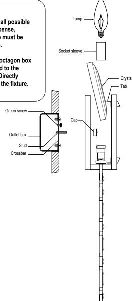
4. Fasten the white fixture lead to the white wire in the outlet box. Fasten the wires together with an approved fastener (wire nut). Starting about 1" below the fastener, tightly wrap the connection with electrical tape so that the connections seals the end of the fastener.
