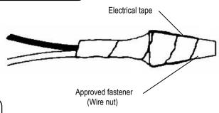
4. Fasten the white fixture lead to the white wire in the outlet box. Fasten the wires together with an approved fastener (wire nut). Starting about 1" below the fastener, tightly wrap the connection with electrical tape so that the tape seals the end of the fastener.
