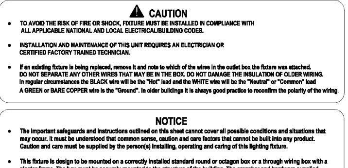
This fixture is design to be mounted on a correctly installed standard round or octagon box or a through wiring box with a plaster frame. The box must be securely mounted to the structure of the building. The crossbar and hardware supplied should be used. Directly mounting the fixture to the outlet box may make it impossible to correctly align the fixture.
