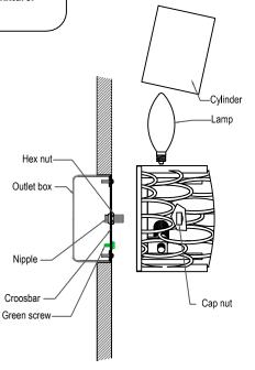
4. Fasten the white fixture lead to the white wire in the outlet box. Fasten the wires together with an approved fastener (wire nut). Starting about 1" below the fastener, tightly wrap the connection with electrical tape so that the connections seals the end of the fastener.
