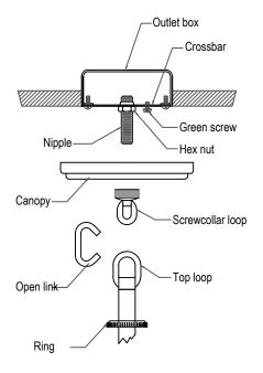
**5.** Using the open link of chain.hang the fixture on the screwcollar loop. Using the chain pliers.close the chain link.
