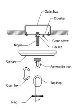
**5.** Using the open link of chain.hang the fixture on the screwcollar loop. Using the chain pliers.close the chain link.
