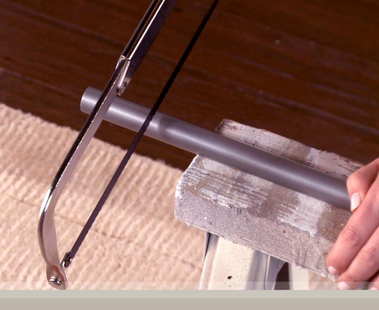
Hang rods may require cutting to fit your closet space. If necessary for smaller closets, measure and cut rod with a hacksaw on the end without a hole.
