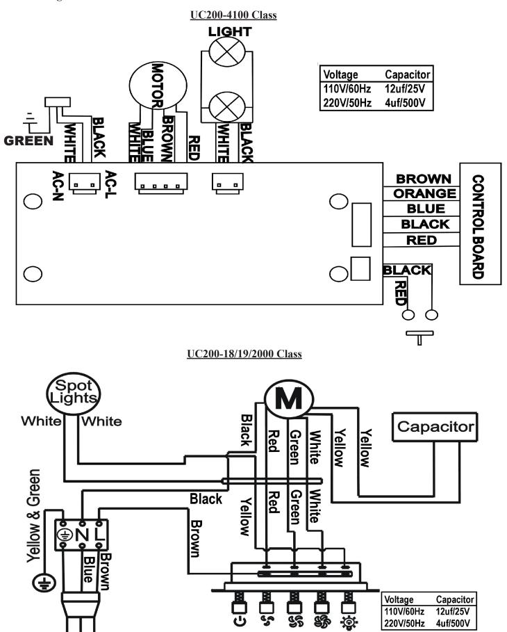
NOTE: Wiring Diagram shown above with GU10 light configuration. A transformer is required for MR16/J4 Lights.
