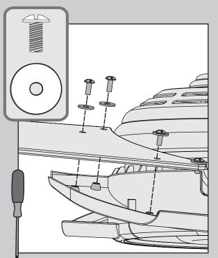
Insert four blade assembly screws and four  $(\mathbf{X})$ blade washers, found in the  $\blacktriangle$  hardware bag, into each blade as shown. Install the screws into the posts in each blade arm.
