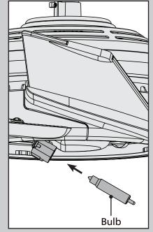
Install a halogen bulb in the light socket. When necessary, replace with bulbs of the same type and wattage.
