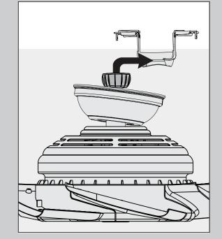
**DO NOT PICK THE FAN UP BY THE CANOPY OR WIRES.** Place the downrod ball into the slot in the ceiling bracket.
