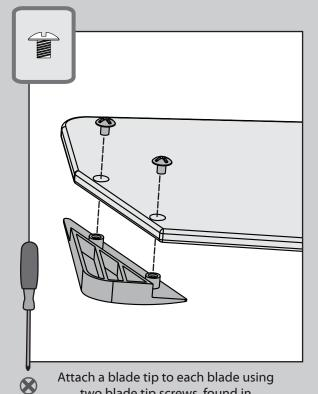
two blade tip screws, found in the  $\blacktriangle$  hardware bag.
