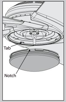
Position the notches in the outer rim of the globe so they line up with the tabs on the inside of the rim on the light kit. Carefully lift the globe up inside the light kit as far as it will go, then rotate the globe clockwise until it is held tightly in place by the four tabs.
