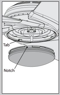
Position the notches in the outer rim of the globe so they line up with the tabs on the inside of the rim on the light kit.
