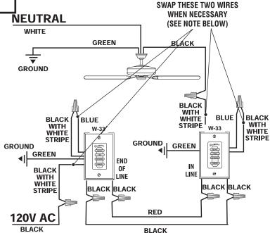
**NOTE:** If wall control operation is reversed (fan switch controls lights and light switch controls fan) <u>turn off the power at the breaker or fuse panel</u>, then swap the two W-33 black/white stripe wires.
