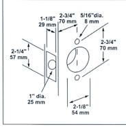
**Door Preparation** When Optional Thru-**Bolt Is Applied**
