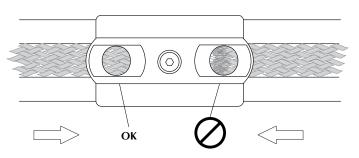
Insert both track ends into connector before tightening thumb screws; the conductive braiding should not be visibly frayed or protruding through the screw hole (arcing and overheating may result).
