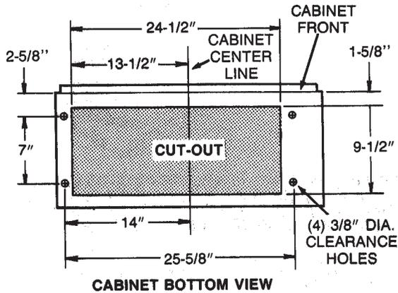
Prepare the cabinet bottom as shown above. Be sure to locate the cut-out and four holes from the front of the cabinet to assure a flush mount.
