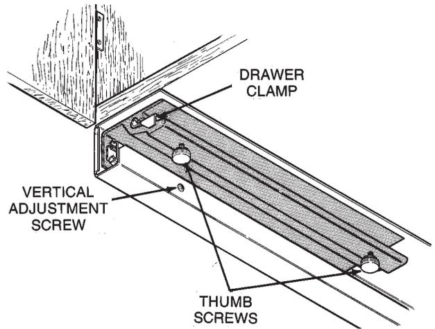
The drawer slides each have a screw for adjusting the height of the drawer trim, if necessary. The vertical adjustment screw allows the top and bottom edges of the drawer trim to be matched with the control trim.
