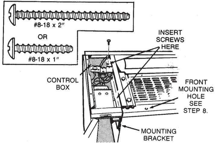
Insert two (2) screws, short or long as appropriate, through control box and into other mounting bracket. Do not tighten screws completely.
