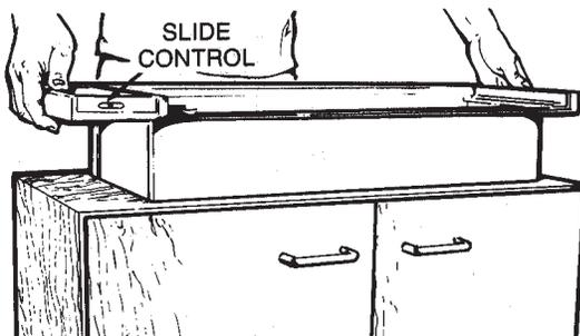
Carefully lower housing into cabinet opening with slide control to the front.
