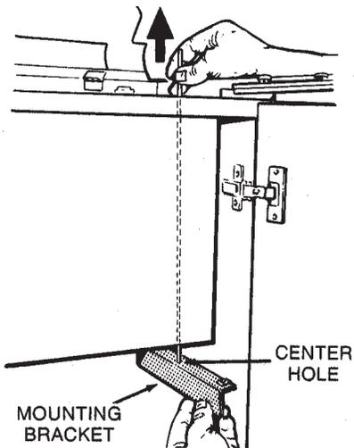
Choose the mounting bracket with the center hole. Hang the bracket from the rod, through this center hole, as shown. Pull bracket up between cabinet and housing.
