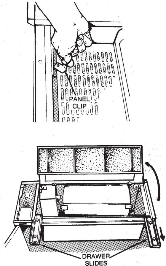
Pull drawer slides out. Rotate panel clips and swing panel open.
