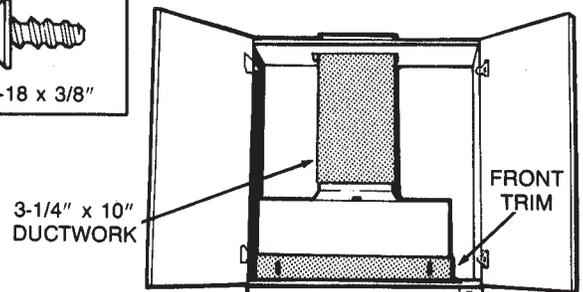
Complete the ductwork from the hood, to the outside, using a roof cap or elbow and wall cap. Tape all joints. Shelves may be installed if trimmed to clear ductwork.
