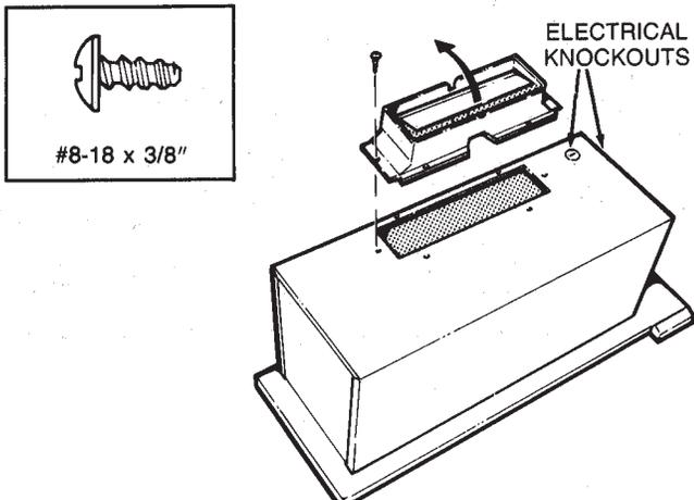
Use two (2) screws (provided) to attach connector to housing. Damper flap should open in direction indicated by arrow.
