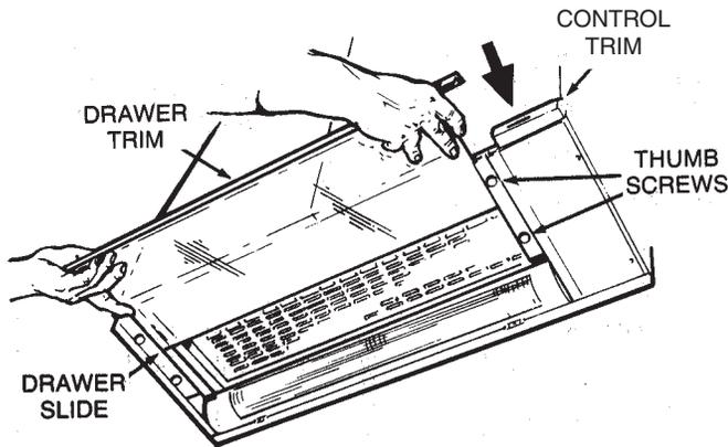
Slide the glass into the drawer slides, above each drawer clamp (see illustration in Step 14). Align drawer trim and tighten thumb screws to secure drawer.
