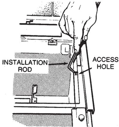
Insert bent end of installation rod into access hole in housing.
