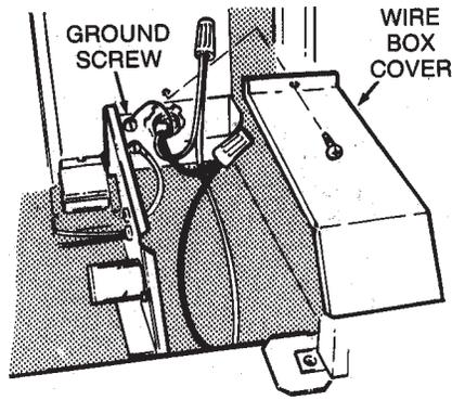
Remove the wire box cover. Attach power cable to hood using proper connector. Connect black to back, white to white and green or bare wire to ground screw. Replace wire box cover.
