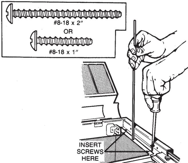
Hold mounting bracket in place with rod. Two sets of screws are provided. Use short screws for flush bottom cabinets or long screws for recessed bottom cabinets. Insert two (2) screws through housing and into mounting bracket. Do not tighten screws completely.
