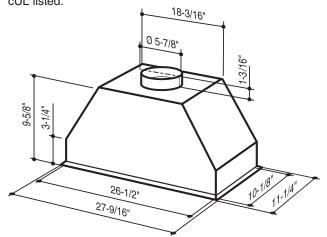
Mount power pack so bottom of unit is 24" to 30" above cooking surface.
