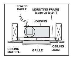
Housing mounted anywhere between trusses using mounting frame.
