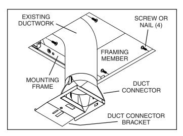
4. Snap the duct connector onto the duct connector bracket. Retrieve the existing ductwork from above the ceiling and connect it to the duct connector. Tape the connection. NOTE: Existing rigid ductwork will require a short length of 4" flexible duct. Existing 3" ductwork will require a 3" to 4" transition.
