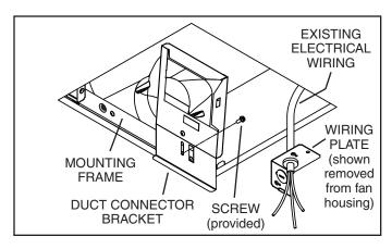
5. Attach the duct connector bracket to the mounting frame using the (1) screw provided. Position the bottom edge of the duct connector bracket so it touches the finished surface of the ceiling and tighten the screw.
