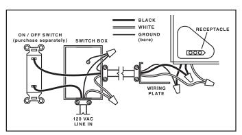
Retrieve the existing electrical wiring from above the ceiling and use a UL approved connector to secure it to the wiring plate. Re-attach wiring plate to fan housing, if necessary. Connect wires as shown in wiring diagrams.
