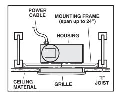
Housing mounted anywhere between standard joists using mounting frame.
