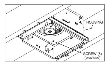
3. Position the two movable brackets of the mounting frame directly across from each other and insert the housing into the mounting frame until it touches the duct connector bracket. Secure the housing to the mounting frame and duct connector bracket using the (5) screws provided. Position the housing horizontally as desired.
