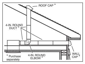
The unit will operate most quietly and efficiently when located where the shortest possible duct run and minimum number of elbows will be needed.
