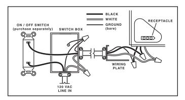
Run 120 VAC housing wiring to installation location.
