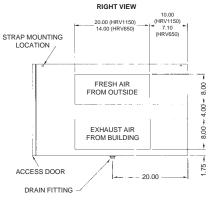
NOTE: These models have a damper located on the outdoor intake connection. This damper will close in defrost or when the unit is placed in the "off" position with power maintained to the unit. This damper is not designed as a backdraft damper and will remain open if power is disconnected to the unit for any reason.
