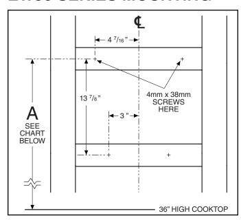
Construct wood wall framing that is flush with interior surface of wall studs. Make sure the framing is centered over installation location.
