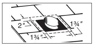
Trim shingles as shown, so they will fit snugly around hood of roof cap when installed. Seal all around duct with roof cement.
