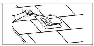
4. Lay roof cap over ductwork and trace outline of roof flange onto shingles.
