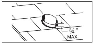
3. Trim ductwork parallel to roof pitch.
