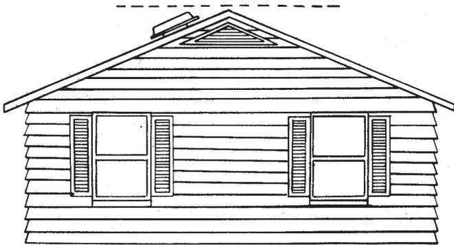
1. Locate the ventilator at the center of the rear slope of the roof. Place it as high on the roof as possible. The location should be free of obstacles (T.V. leads, electrical lines, etc.) If the ventilator top is level with the roof peak, it can't be seen from the street. Keep this approximate location in mind as you work from within the attic.
