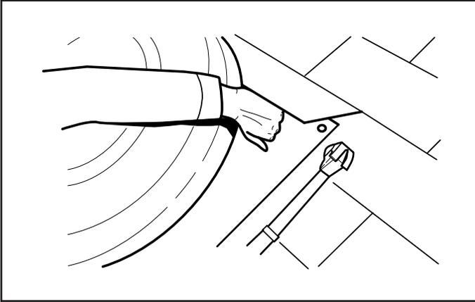
12. Carefully lift shingles and nail flashing securely to the roof using galvanized roofing nails.
