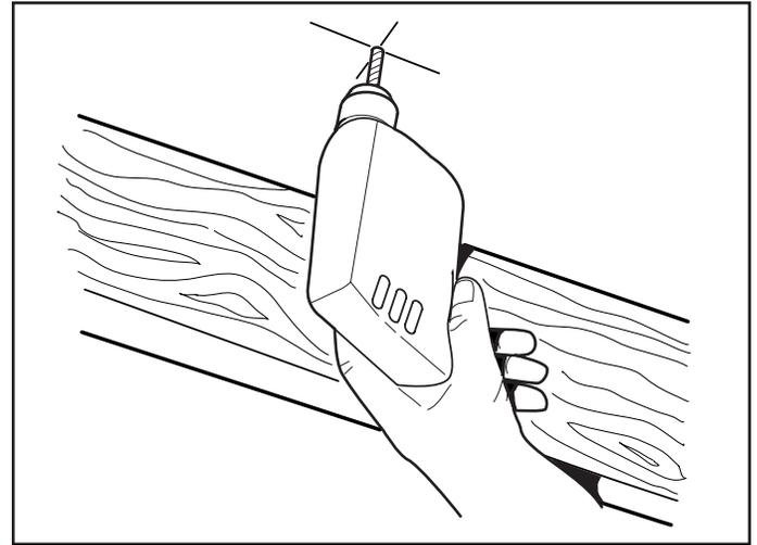
3. Drill a guide hole through the roof at this mark.
