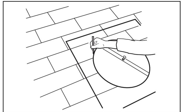
5. Push a large nail through the center of the cardboard template and into the guide hole.
