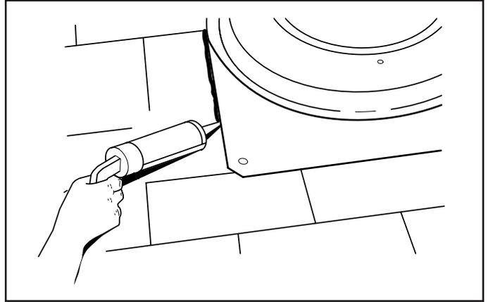
13. Using a good grade of roofing cement material, seal all of the shingles and heads of nails.
