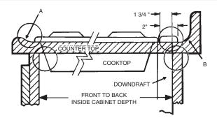
Refer to the cooktop installation instructions for dimensions of cooktop, countertop cut-out, and cabinet requirements. The 2730 and 2736 can be installed in most standard 30" and 36" wide cabinets.
