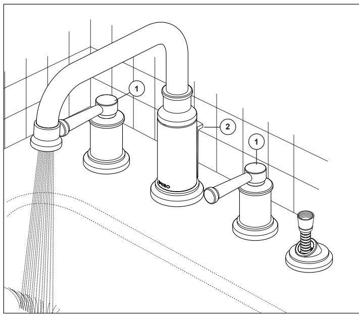
Make sure the finial (2) is in the down position. Turn faucet handles (1) all the way on. Turn on hot and cold water supplies and flush water lines for one minute. **Important: This flushes away any debris that could cause damage to internal parts.**
