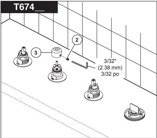
**NOTE:** The deck and valve rough-in (R62707, R64707) must be installed before installation of the trim kit begins.
