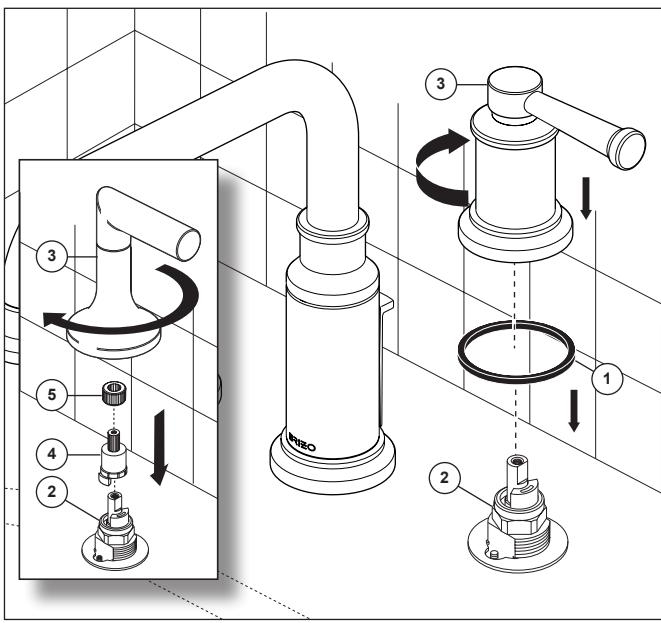
Place gasket (1) over valve assembly (2). Make sure valve stem is in the off position. Align and place handle (3) over valve stem and onto base. Make sure handle is properly seated. Turn handle base clockwise until surely tighten. Repeat for other handle.
