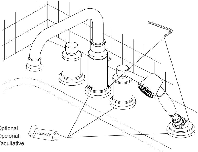
"The Commonwealth of Massachusetts requires all hand-held shower sprays to comply with the Massachusetts State Plumbing Code 248 CMR whereby their installation shall include a device that limits the maximum deliverable temperature of hot water to 110°F and an approved backflow prevention system."
