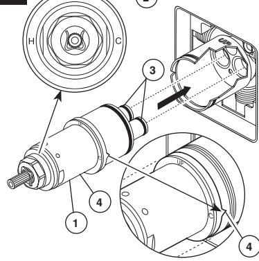
Rotate the cartridge (1) so the word "UP" (2) appears on the top. Insert cartridge into valve body as shown. Make sure the cartridge tubes and O-rings (3) are properly seated in holes at the base of the body. Ensure the keys on the body are fully engaged with the slots in the body (4).
