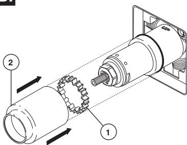
If your model requires a spacer (1), install it into sleeve (2). Slide the sleeve over the cartridge, body and O-ring. Ensure sleeve is properly positioned over the front of cartridge. **Note:** RSVP™ models (series T60X90) do not require spacer (1).
