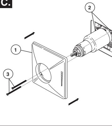
Secure the escutcheon (1) to the bracket (2) with the 2 screws provided (3). Do not overtighten escutcheon screws.
