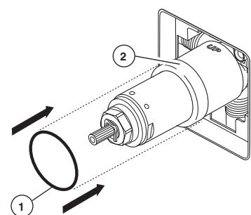
Slide O-ring (1) over cartridge and the bonnet (2). The O-ring, which acts as a spacer to steady the sleeve, should rest behind the bonnet nut.
