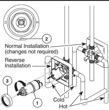
For back to back or reverse installations (hot on right and cold on left): Rotate cartridge (1) so the word "UP" (2) appears on the bottom. Install the cartridge making sure that the keys are fully engaged with the slots in the brass body (see step B). Slide bonnet nut (3) over the cartridge and thread onto the body. Hand tighten securely.
