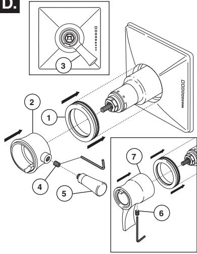
Slide trim ring (1) over the cartridge and sleeve and into the escutcheon. Install volume control handle base (2) with lever to the right as shown (3). Install set screw (4) followed by the handle lever (5).
