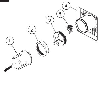
**Turn off water supplies.** Remove cover (1), bonnet nut (2) and test cap (3) from the body. If this is not a thin wall mounting, the entire plas-terguard (4) may be removed. If screen (5) is in place, remove before installing cartridge.
