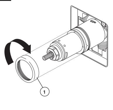
Slide bonnet nut (1) over the cartridge and thread onto the body. Hand tighten securely.
