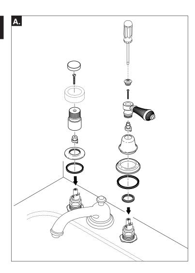
Using silicone sealant (1) under the spout (2), install the spout on the spout adapter (3). Be sure the spout is resting firmly on the deck
