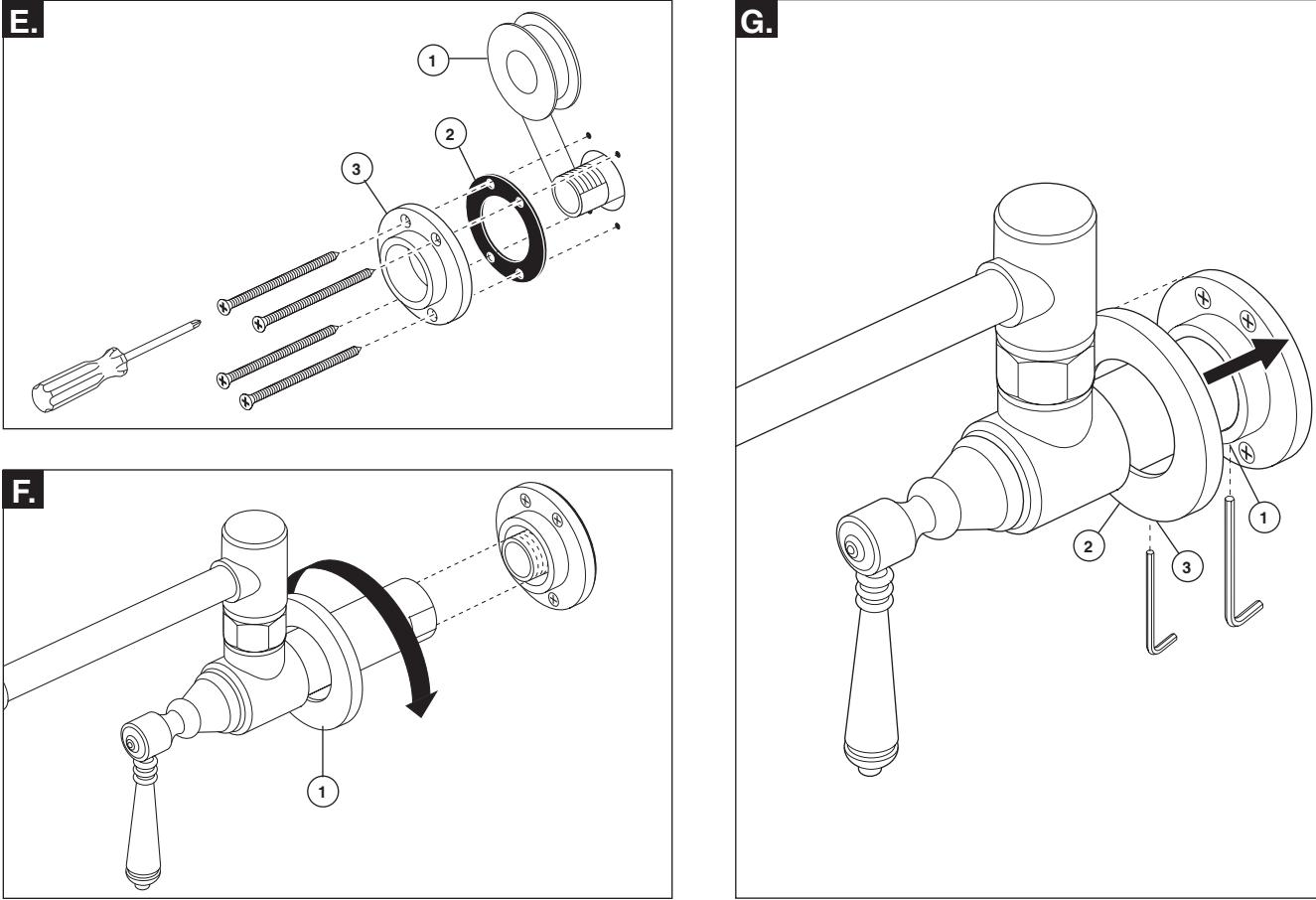
**E.** Wrap Plumber tape (1) around pipe threads. Install the gasket (2) and the flange (3) using the 4 screws (and anchors if required) provided.
