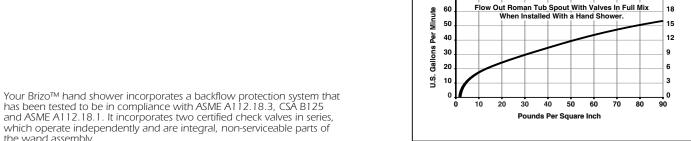
and ASME A112.18.1. It incorporates two certified check valves in series, which operate independently and are integral, non-serviceable parts of the wand assembly.
