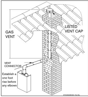
Fig. 11 Masonry chimney
