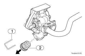
Fig. 24 Drain plug and filter location
