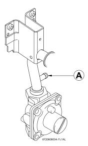
Fig. 13 Gas pressure measuring point
