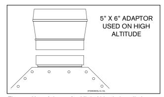
Fig. 9 Vent Adaptor for High Altitude Installations
