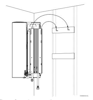
Fig. 7 Secure heater to wall
