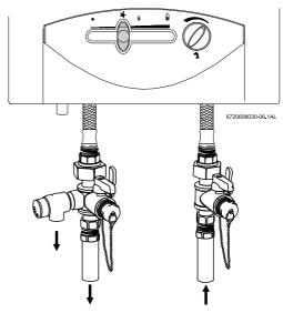
Fig. 14 Plumbing connections and pressure relief valve shown with optional Webstone service valves
