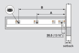
Mount each runner using at least two of the elongated holes. Install the drawer to check the position of the drawer front.
