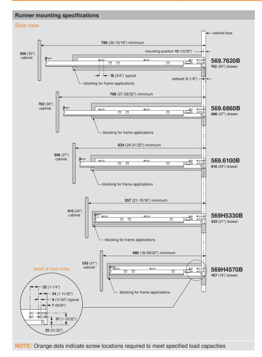
Cabinet and drawer specifications Side view cabinet depth inside cabinet depth cabinet face runner length mounting position 10 (13/32") -37 (1-15/32") **25** (31/32") setback 3 (1/8") blocking behind frame minimum top clearance 6 (1/4") drawer length maximum drawer height = opening minus 20 (25/32") bottom clearance 14 (9/16") drawer gap 1.5 (1/16") blocking behind frame drawer thickness 000 bottom recess 13 (1/2")
