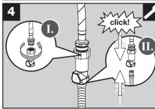
Attach hose connector (17) to the supply line (15). Connect spray hose (12) to supply line (15) by inserting end of spray hose into the hose connector until it clicks into place.
