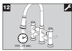
Open the water levers and flush for at least 20 seconds the lines and the faucet.
