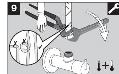
Connect red supply line (16) to hot water valve and blue supply line (19) to cold water valve.
