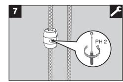
Attach weight (18) to spray hose using screws provided.
