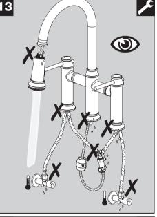
Double check all connections for leaks.
