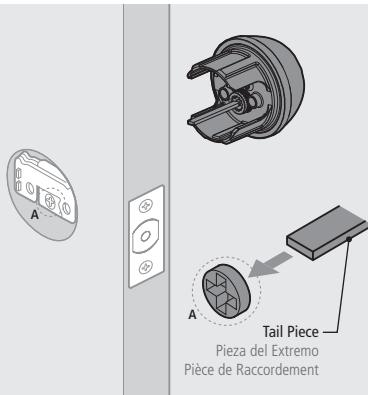
Mount turnpiece assembly on door, aligning onto tail piece. Insert screws, engaging the exterior assembly. Tighten screw firmly to secure assemblies to door.
