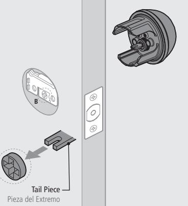
Mount interior cylinder assembly on door, inserting tail piece into latch crank at a vertical position. Insert screws to engage exterior assembly and tighten securely.
