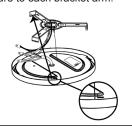
9. Attach fixture to bracket arms by twisting the fixture clockwise. Make sure fixture is secure before turning on power at source.
