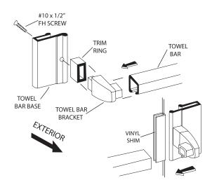
Align the two pull handles [R] and vinyl shims [P] into place on the interior glass panel at the same height as the towel bar bases [L] were mounted on the exterior panel.
