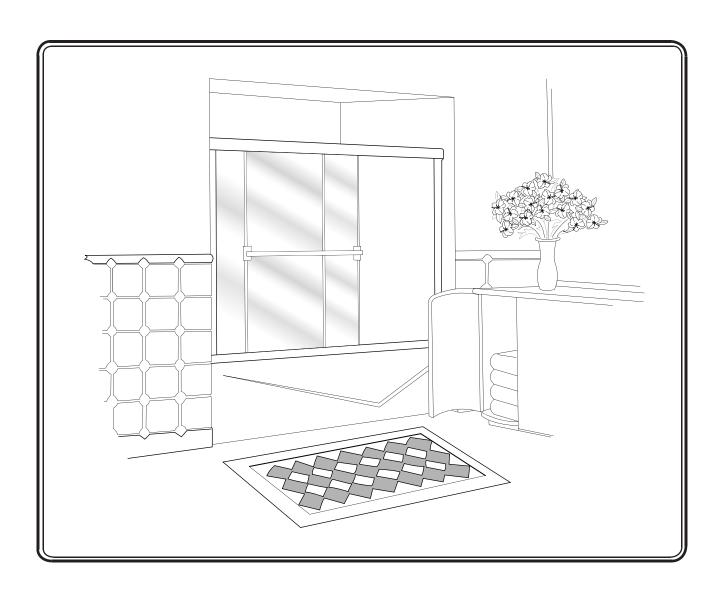
**MAINTENANCE:** Two primary materials are used to manufacture your new enclosure: tempered glass and anodized aluminum. To assure a long lasting finish on the enclosure, wipe it down with a towel after each use. Never use a scouring agent to clean the aluminum.
