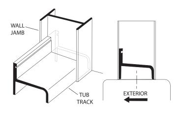
**2**Use a level to plumb both wall jambs [B], then mark the pre-drilled hole locations on the wall. Lightly mark along both sides of the tub track [A] with a pencil, then remove all parts.
