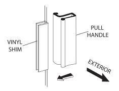
Before installing the door panels, the proper orientation should be determined. For maximum water-proofing, the interior panel should always be positioned closest to the shower head, as shown in this illustration.
