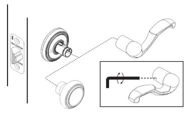
Place lever or knob onto assembly and tighten set screw to secure. Repeat for the knob or lever on the other side.
