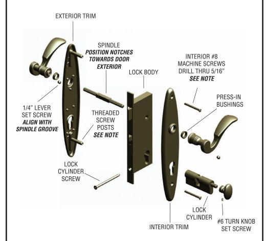
**#8 Machine Screws Note:** Proper trim alignment requires installing the spindle and levers before completely securing the #8 screws.
