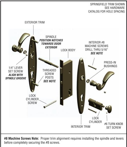
**Threaded Screw Posts Note:** Length may need to be cut down to accomodate different door manufacturers' hole pattern.
