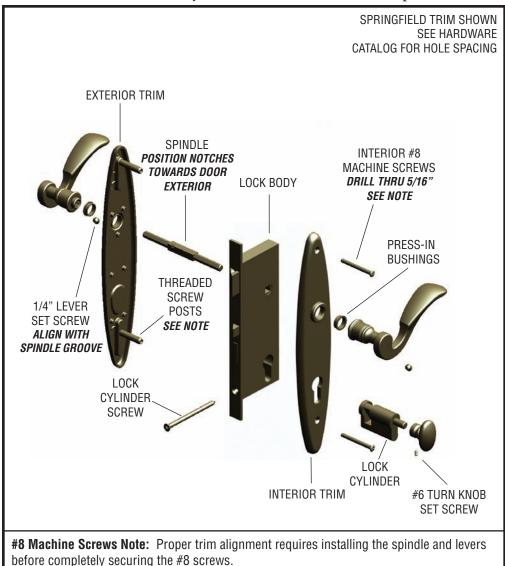
**Threaded Screw Posts Note:** Length may need to be cut down to accomodate different door manufacturers' hole pattern.
