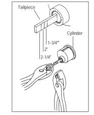
6 Align tailpiece with slot. Keep tailpiece vertical and curved towards right side of the hole as illustrated.
