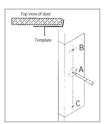
Drill a 2-1/8" diameter face bore (A). Drill the 1/2" dummy cylinder hole (B) through the door. Drill the 5/16" lower pull assembly hole (C) for the appropriate handleset shown on template.
