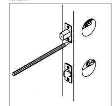
Chisel out area marked in step 3 to a depth of 5/32" or until faceplate is flush with door edge.
