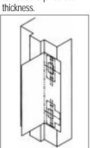
2 Align and trace the outline of strikes onto the door frame using mounting screw marks for location.
