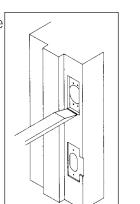
trace an outline of the faceplate onto the door edge. Mark screw hole centers and drill. Remove deadbolt and repeat process
