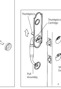
Hold outside handle assembly in place. Attach adaptor with the short #10-32 x 2-1/8" truss head screw in the top hole and the long #10-32 x 2-5/8" truss head screw in the bottom hole. To secure bottom of outside handle, insert the #10-32 x 2-1/2" flat head machine screw through the screw cover backplate. Screw through door and into bottom of outside handle. Tighten all screws.
