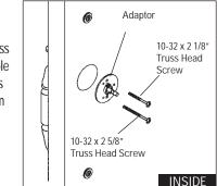
Snap rosette onto adaptor. Slide knob onto spindle and tighten set screw. Attach screw covers. Congratulations! Your installation is now complete!
