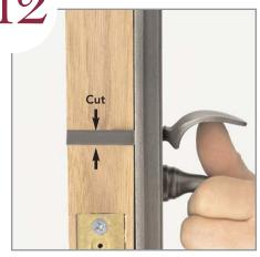
Cut the thumbpiece so that it will fully engage the lift lever on the bottom of the lock.
