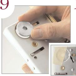
Thread the cylinder plug into interior side of lock. Place a strip of tape over plug to keep it from turning. Notch must be located as shown. (Double cylinder functions: OMIT THIS STEP.)
