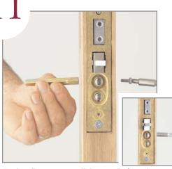
For handleset trim install the spindle from the inside with V groove facing bottom door hinge and thread the screw and lock washer into the spindle from the outside. Tighten securely. For knob to knob and lever to lever sets, install spindle from outside - go to step 13.
