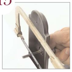
Cut the thumbturn tailpiece so that it goes halfway through the lock (as in step 12).
